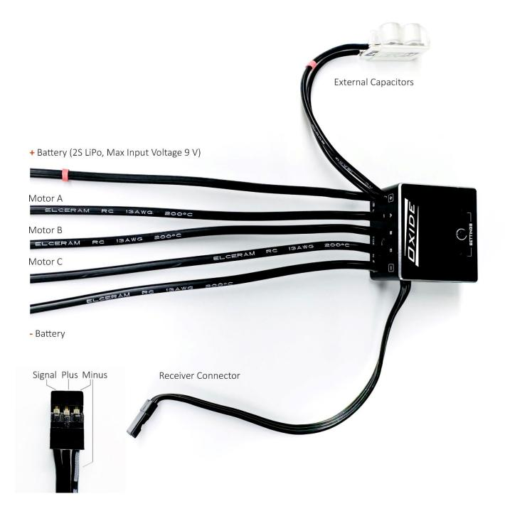
! WARNING! Please, double check the polarity of battery interconnection! Make sure, that positive (+) of ESC is connected to the positive (+) of battery. If polarity is reversed, the ESC will be damaged!
