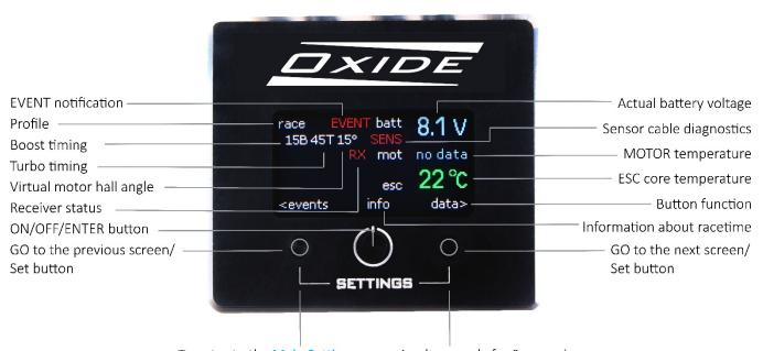
To enter to the Main Settings press simultaneously for 2 seconds.
