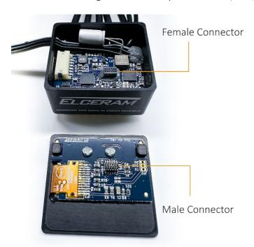
Please be informed, that the cover with display and buttons is replaceable in case of any incident – spare part number ELC002.
